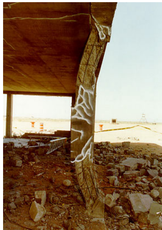
(c) Response observed in DB 6 blast test.
