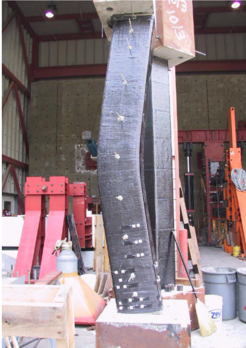
Figure 3. Column with good confinement having support rotation, around 10^\circ rotation.
