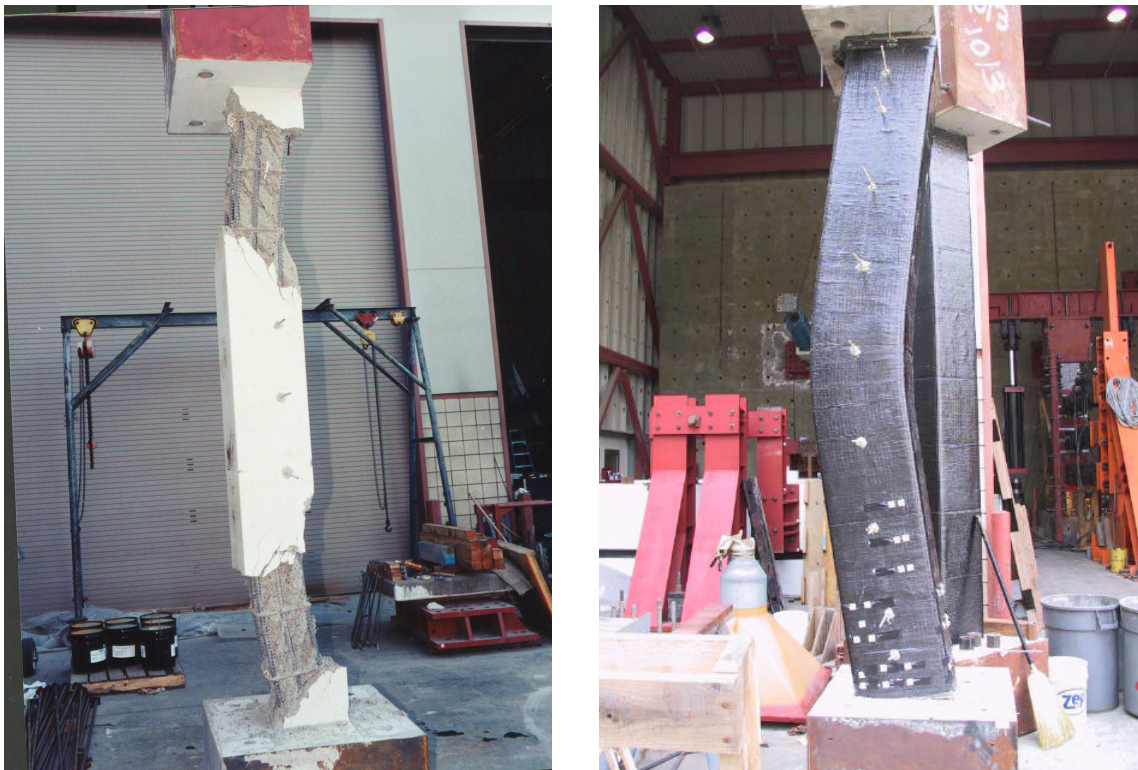
Figure 22. Composite wrap for reinforced concrete column, converting brittle blast response of column to highly ductile one.
