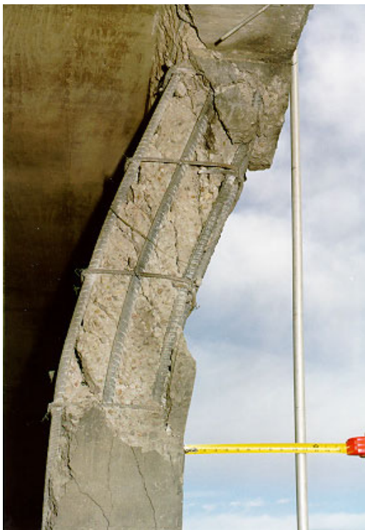
(c) Response observed in DB 6 blast test.
