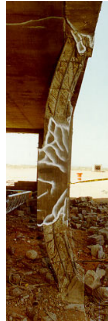
(b) CTS-1 test structure, a flat slab design for an area of low seismicity; center first-floor column (shown to right) was destroyed by blast.
