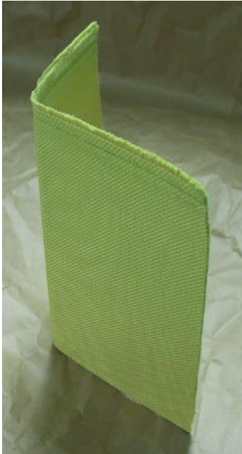
(a) Kevlar laminate, provided in multiple plies (10 plies = 17,000 lb/in capacity).
