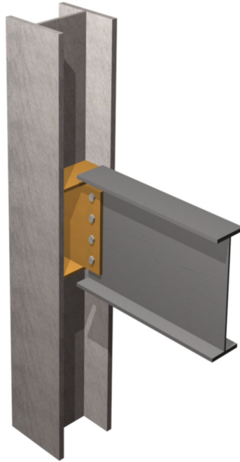
(c) Conventional bolted shear connection, weak axis.
