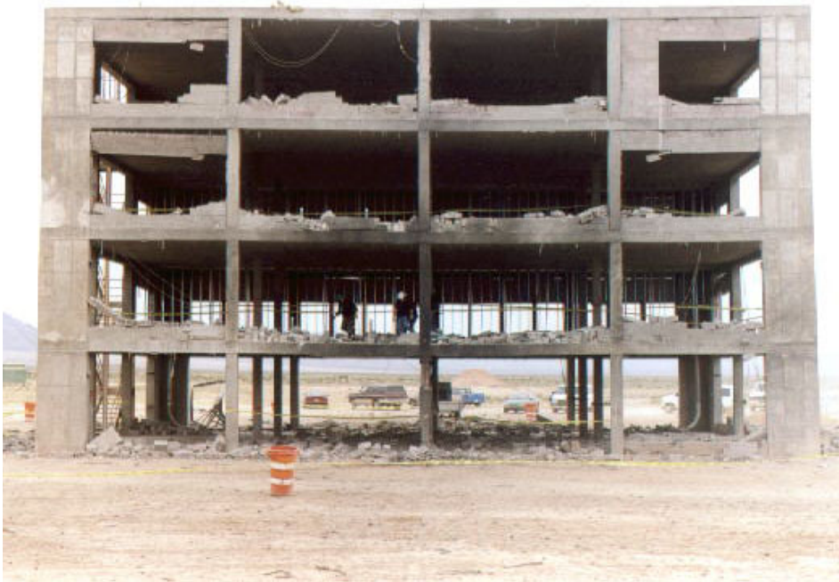
(b) CTS-1 test structure, a flat slab design for an area of low seismicity; center first-floor column (shown to right) was destroyed by blast.
